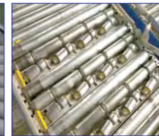
Steerable rollers can change the direction of delivery of goods
