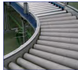
Turning section The difference in speed on either side of the conical roller to rotate the object with it.
